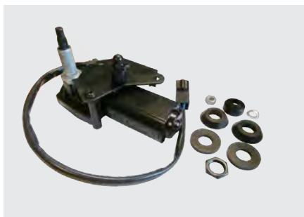
63240 Massey Ferguson Wiper Motor Front 54s 42s 43s - mounted
