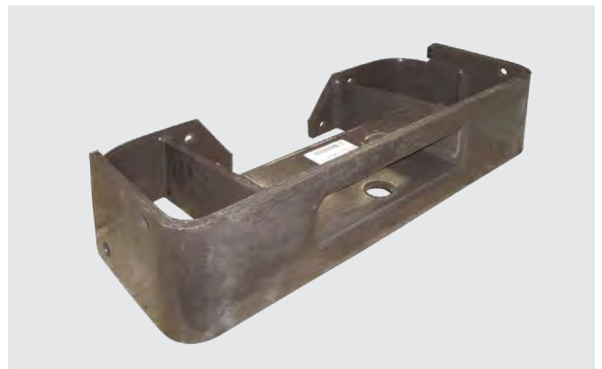
3541 Massey Ferguson Weight Carrier 135 240 - Straight Axle Bolt to suit is 353728 OE Ref: 1673901M91
