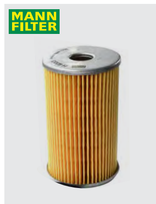
H820/3X Engine Oil Filter 35 135 Paper 114mm Long 71mm OD OE Ref: 1851766M1
