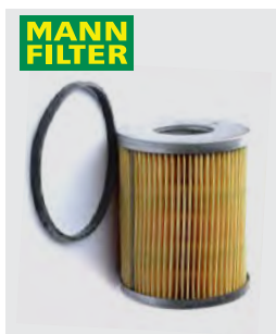
P824X Fuel Filter 35 65 100 Series Length: 82.5 OD: 71.00 ID: 33.5 OE Ref: 1850450M1
