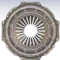
4260 Clutch Assembly Same Explorer 12"
